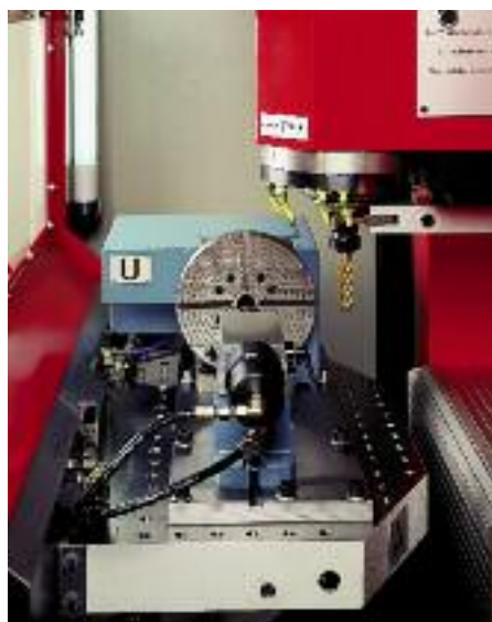
Working area with mounted CNC rotary table and tail stock
