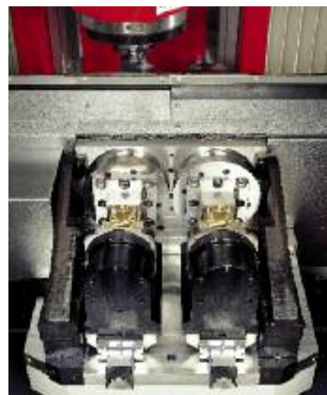
Loading station with 2 CNC rotary tables and clamping device
