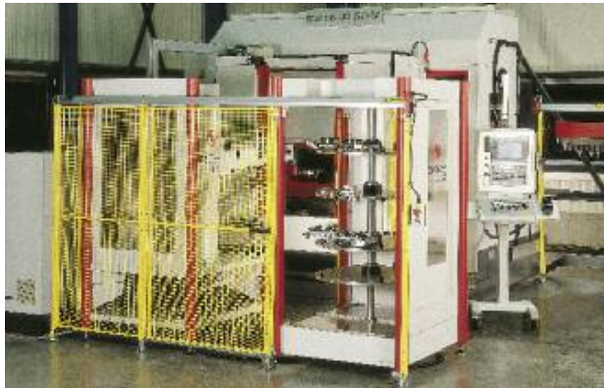
Machines can be tailored for special purpose applications, e.g. multiface machining with additional tools and pallet storage
