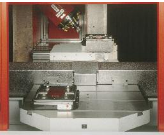
Working area matec-30 SHV Station 1: CNC rotary table with EROWA pallet system Station 2: stationary EROWA pallet system
