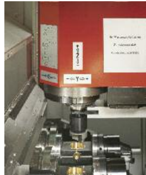
Working area with 2 CNC rotary tables, clamping device and machining tool
